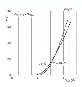
$T_j = 25$ °C and 175°C; $V_{DS} > I_D \times R_{DSon}$
